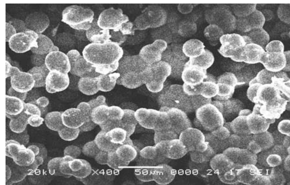
Fig. 6 Scanning electron microscopy (SEM) photograph of pure PVDF
